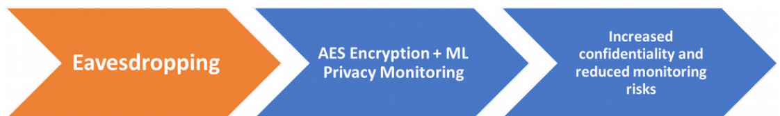
Fig 6 | Threats and hybrid solutions for ADS-B security-eavesdropping
