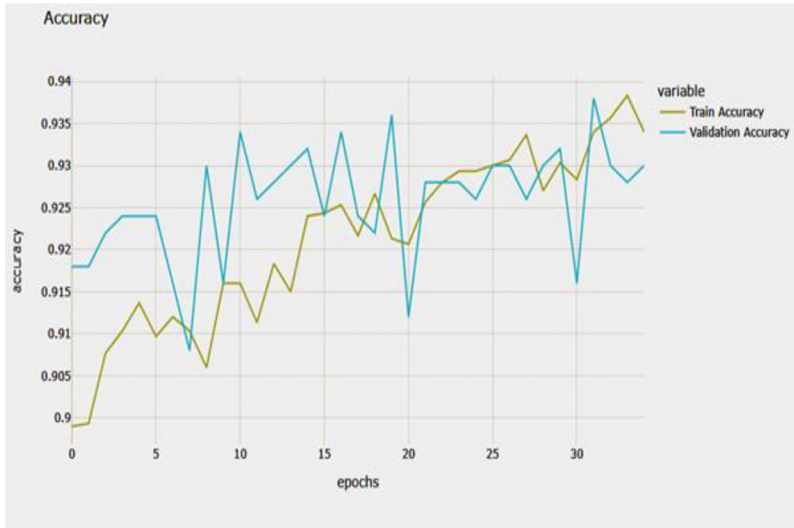
Fig 2 | Training and validation accuracy curves of the MobileNetV2 model over 32 epochs. Training accuracy rose steadily, reaching 93.4% at the final epoch, while validation accuracy fluctuated slightly
